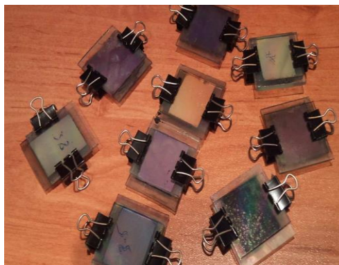
Figure 1: The picture of some of the manufactured dye sensitized solar cell (DSSC) in this study.
