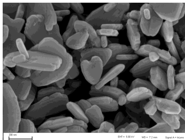
Figure 1: Figure illustrating the SEM micrographs of the samples synthesized with H_2O
