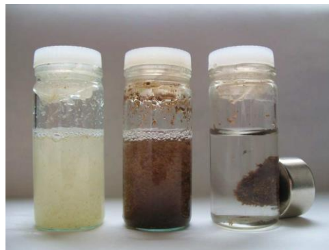
Figure 1: Appearance of original sawdust suspension (left), suspension of sawdust after magnetic modification (middle) and demonstration of magnetic separation of magnetically modified sawdust (right) (Safarik et al., 2013).
