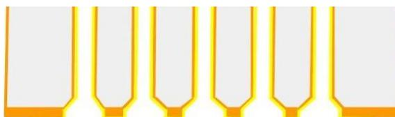
Figure 6: Barrier material deposition. This leads to stop the copper atoms diffusion and limits the parasitic copper growth on the sidewalls of silicon.
