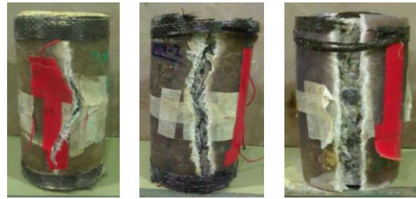
vertical rupture      partially inclined      inclined ruptures
