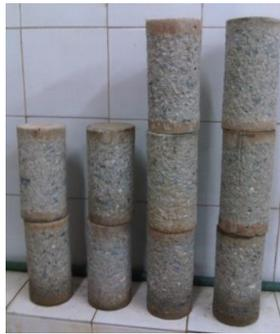
Figure 1: Typical roughened surface of specimens
