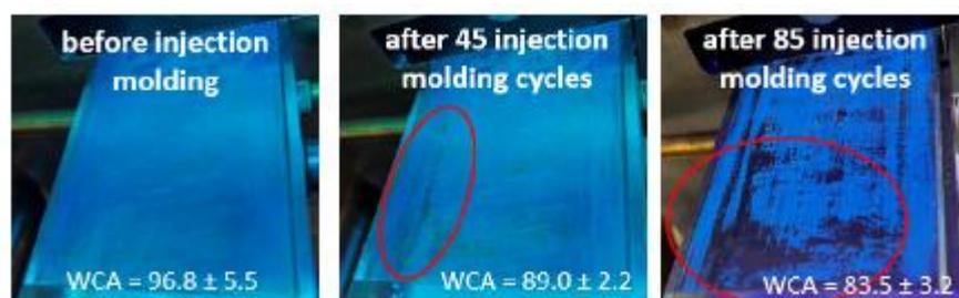
**Figure 3:** NIPTES containing coating along injection molding experiment
