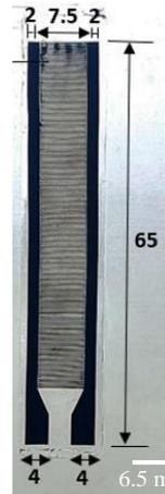
Fig. 1: Capacitive strain gauge sensor. [6]
