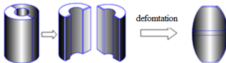
Fig. 2 Samples' obtaining and deformation scheme
