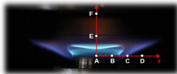
Fig. 1: Impinging premixed flame with equivalence ratio ( \phi ) = 1,6 and reynolds number (Re) = 300. Coordinates (x, y) in millimeters: A = (0, 0); B = (6.5, 0); C = (13, 0); D = (19, 0); E = (0, 10); F = (0, 20).
