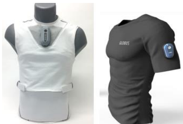
Figure 3: Examples of smart textile prototypes. Left a stress monitoring vest with off-the-shelf, rigid sensors and copper interconnection wires; Right a posture monitoring fitness shirt with textile based sensors [8]
