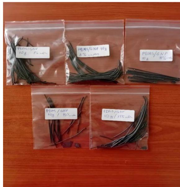
Fig. 4. Filaments of graphene/polymer composites made by extruder
