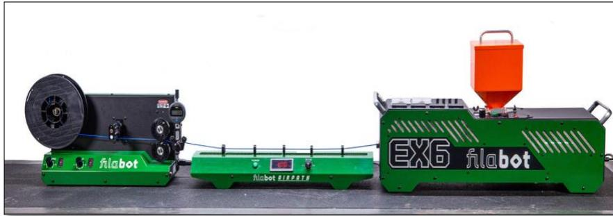
**Fig 1.** Extruder for the production of polymer threads
