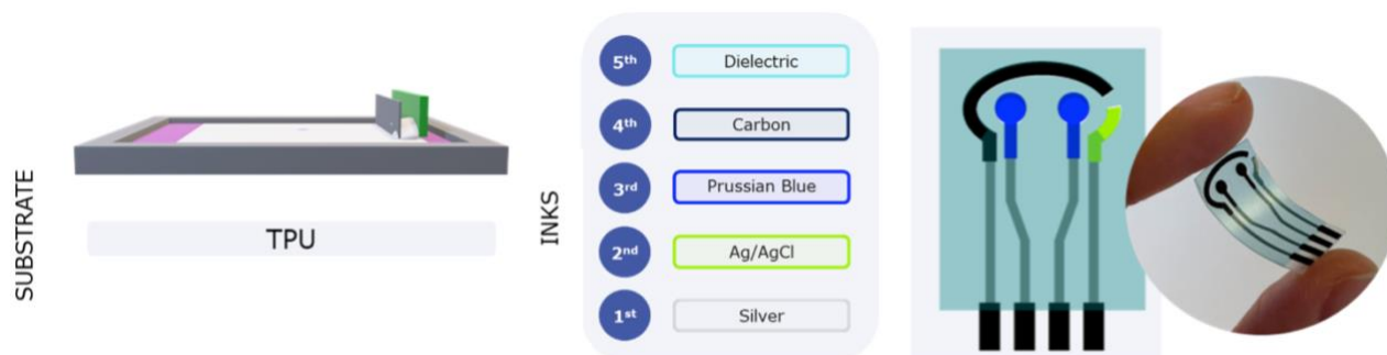
Fig. 1: Schematic representation of the different printed layers in TPU and the resulting screen-printed electrode
