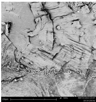
Figure 4. Damaged inner surface of the scaffold of PCL in formic acid solution. (Scale bar 400x)
