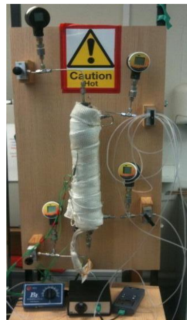
Figure 5: Membrane's Heat-Treatment Profile. Figure 6: Stainless Steel Tubular Membrane Reactor.
