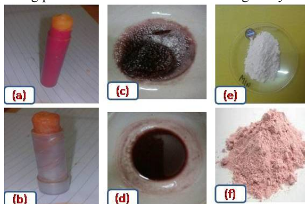
Figure 2 (a) Lipstick made using iron oxide, (b) lipstick made using iron oxide nanoparticle, (c) sunscreen made using iron oxide, (d) sunscreen using iron oxide nanoparticle, (e) talcum powder made using iron oxide and (f) talcum powder iron oxide nanoparticle.
