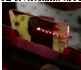
Figure 1: Slanted transmission mode sol-gel HOE waveguide probed at Bragg angle.
