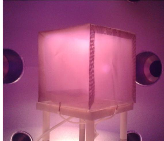
**Figure 1:** Illustration of an inverted fireball (IFB) setup in a low pressure PECVD chamber with a DC argon plasma.
