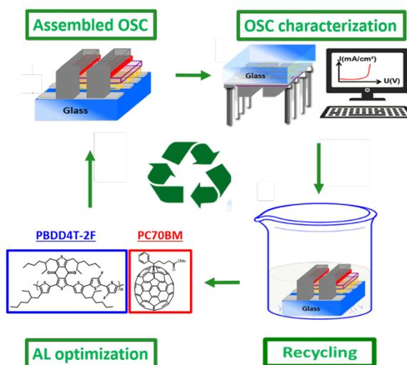
**Figure 1:** Figure illustrating the successful replacement of unstable PEDOT:PSS with CuCrO<sub>2</sub> thin films out of stoichiometry. The assembled cells are electrically characterized. Then, a simple chemical approach is used to recycle the substrate/electrode/HTL structure, allowing the test of different Active Layers and the conception of new cells, finally, enhancing the performances.
