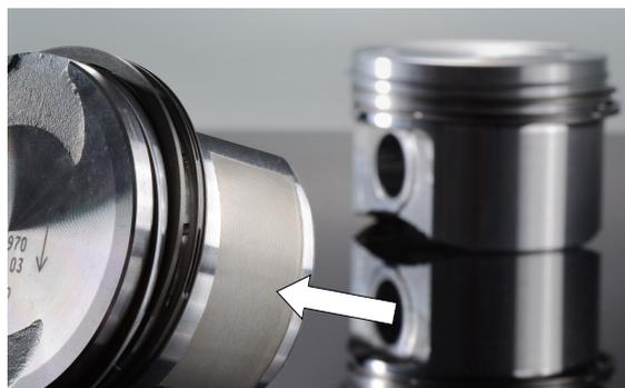
**Figure 1:** Figure illustrating a polymeric tribological coating on an engine piston produced in a laser-based process. The PEEK-based coating can significantly reduce the friction between pistons and cylinders compared to state of the art bonded coatings.
