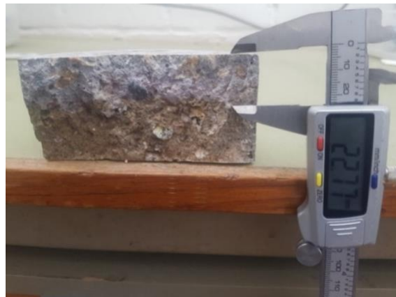
Figure 1: Figure illustrating measuring the chloride penetration depth in a concrete disk as part of the rapid chloride migration test.
