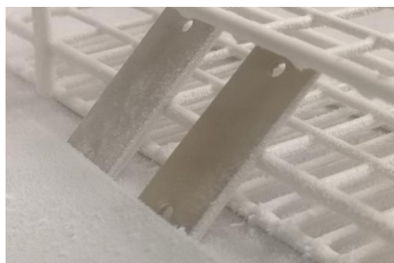
Figure 1: Figure illustrating the static anti-icing tests on the pristine (left) and icephobic (right) polymeric coatings.
