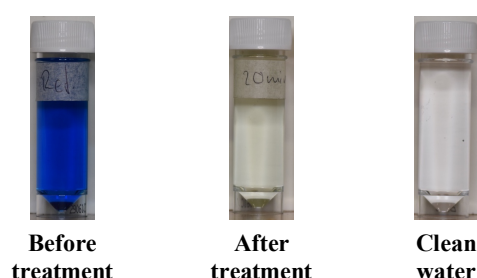
Figure 2. Pictures of treated water samples using a plasma activated microbubbles, where methylene blue (MB) has been used as a simulant of chemical contaminants.
