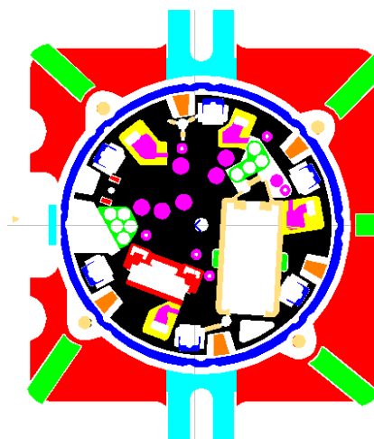
Figure 2: Topographic map of one part of the mould, where the different colours represent different heights planes.
