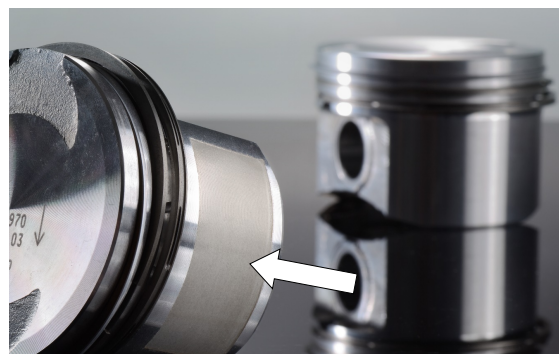
Figure 1: Figure illustrating a polymeric tribological coating on an engine piston produced in a laser-based process.
