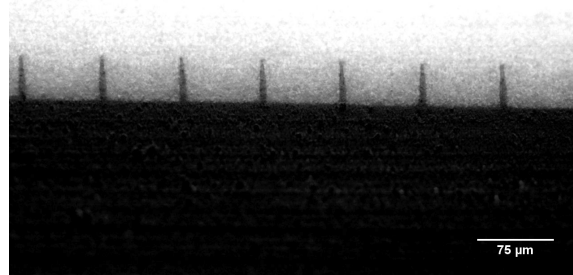
Figure 1: Optical micrograph of the cross-section of the improved riblet structures from PDMS moulded copy of the riblets. These are riblets with spacing 78 \mu\text{m} , height 41 \mu\text{m} , width 7 \mu\text{m} , peak radius 0.8 \mu\text{m} .
