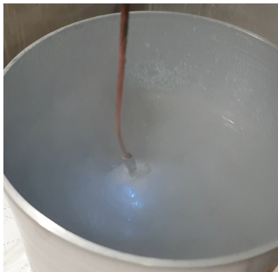
Figure 1: Plasma discharges (blue) on the surface of a stainless steel substrate during the cathodic plasma electrolytic deposition process.
