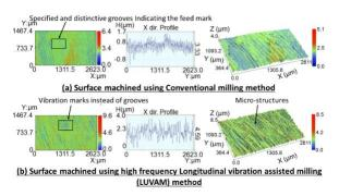
Figure 1: Surface morphology of machined surfaces
