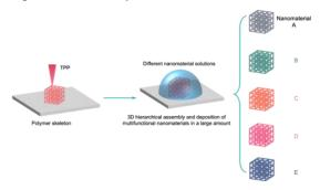
**Figure 1.** Schematic of multifunctional 3D nanoprinting via assembly and deposition of nanomaterials onto polymer skeleton.
