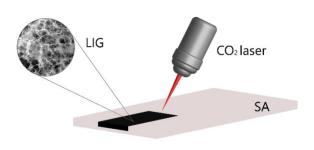
**Figure 1**: Graphene induction onto a sodium alginate precursor with a carbon dioxide laser.
