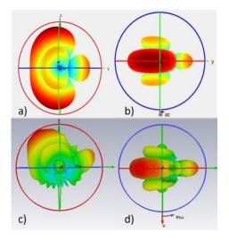
**Figure 1**: Array factor designed to point at Phi = 270 and Theta = 15, and the simulated results. A) and b) represent the array factor, while c) and d) are the corresponding simulated radiation diagrams.
