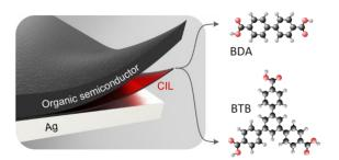
**Figure 1**: Schematic overview of OS device with implemented CIL based on carboxylic acid molecules (BTB or BDA).
