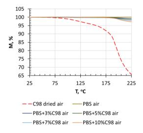
**Figure 1**: Figure demonstrates no considerable changes in thermogravimetric M(T) relationships of PBS composites with various concentrations of LMWC (C98) up to 170°C.
