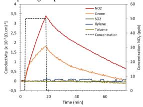
**Figure 2**: Conductivity variations versus time of conductimetric transducer coating by 50nm of CuPc during exposure to various pollutants. For each exposure, microsensor is maintained at 60°C, exposed to pollutants during 15min and then recovered under clean air during 60min. The concentration of all pollutants is 50ppb.
