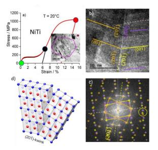
**Figure 1**: Monoclinic B19' martensite in NiTi shape memory alloy deforms via kwinking deformation mechanisms combining [100](001) dislocation slip based kinking with (100) twining. a) stress-strain curve from tensile test at room temperature on nanocrystalline NiTi wire in martensite state. HRTEM image (b) and FFT pattern (c) from (20-1) kwink interface and its atomic model (d).
