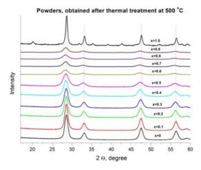
Figure 1: XRD patterns of  $Ce_{1-x}Gd_xO_{2-x/2}$ (x = 0 - 1) powders thetmally treated at 500°C.
