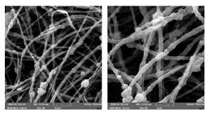
**Figure 1**: Scanning electron microscope images of polycaprolactone polymer with incorporated graphene nanoparticles. Magnification 5000x and 10000x.
