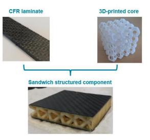
**Figure 1**: Sandwich structured component created from carbon fibre reinforced polymer laminate and 3D-printed lattice core.
