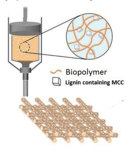
**Figure 1**: Figure illustrating the 3D printing process of honeycomb structure on the wood surface.
