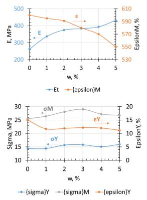
**Figure 1**: Figure illustrates that tensile modulus (E) and tensile strength at yield and strength at break ( $\sigma$ M and  $\sigma$ B, respectively) are increased by increasing the NC content in the PBSA matrix up to certain critical concentration, whereas relative elongation at yield point and elongation at break ( $\epsilon$ M and  $\epsilon$ , respectively) decreases. However, ultimate relative elongation ( $\epsilon$ ) at miximum NC content is 550%.
