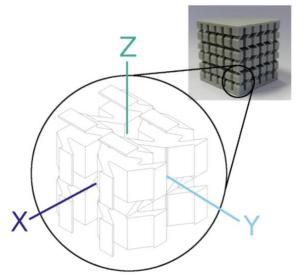
**Figure 1**: Design of a mechanical metamaterial with independently tunable stiffness in the three spatial directions. The stiffness can be varied in the range of several orders of magnitude. Gradual transitions from one unit cell to the next can be realized, enabling smooth transitions from soft to hard regions.
