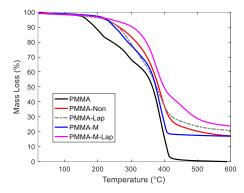
**Figure 1**: TG curves PMMA-Non, PMMA-Lap, PPMA-M and PMMA-M-Lap nanocomposites and the pristine PMMA.
