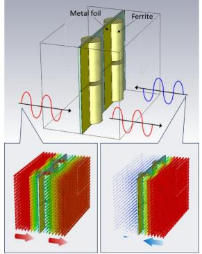
**Figure 1**: The upper figure represents a unit cell analysis model that simulates a pseudo infinite surface,with the proposed structure being represented as 2x2. The lower left part and lower right part show the example of the analysis results in the transmission direction and in the blocking direction, respectively.
