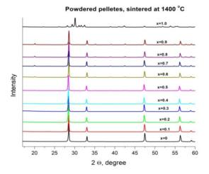
**Figure 2**: XRD patterns of  $Ce_{1-x}Gd_xO_{2-x/2}$ (x = 0 - 1) powders sintered at 1400 °C.
