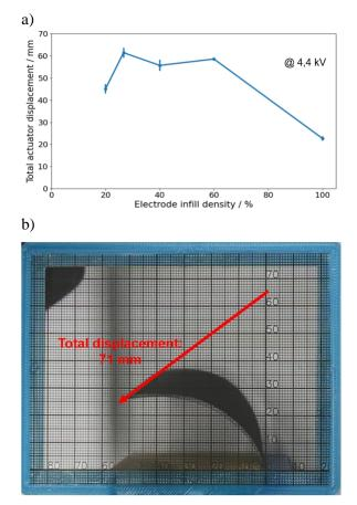
Figure 1: a) The dependence of the electrode infill density to the total actuator displacement.;b) The fully FFF 3D printed DEA reached its maximum displacement.
