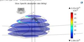
**Figure 1**: SAR levels on a breast heterogeneous model, with acceptable FCC and ETSI values, less than  $1 \times 10^{-3}$  W/Kg (1g).
