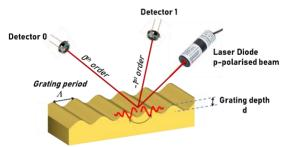
Figure 1: synoptic of SPR gas sensor.
