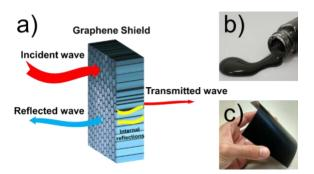
**Figure 1**: a) The exceptional electric conductivity of graphene renders it an excellent material for EMI shielding, enabling the effective blocking incident electromagnetic waves via reflection and absorption of incoming signals.; b) Graphene-based ink for conductive coatings.; c) Extruded G-Shield slab, a conductive polymeric compound designed for EMI shielding applications.;
