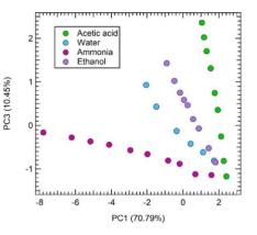
**Figure 1**: 2D PCA space. All tested gases are separated in the space, denoting the good discrimination capability of the developed e-nose.
