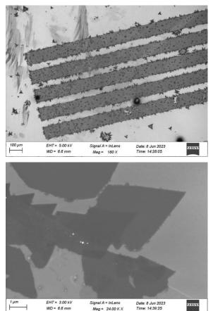
**Figure 1**: (a) SEM image of graphene stipes and darker WS2 triangles growing at the edges of graphene. (b) Enlarge SEM image of the graphene/WS2 junction.
