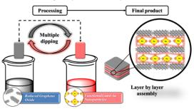
**Figure 1**: Schematic illustration of layer-bylayer processing. **References:**
