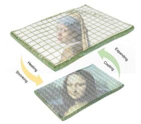
**Figure 1**: Schematics of the reversible thermal actuation of the micro-metastructures displaying dynamically changed encrypted complex information.
