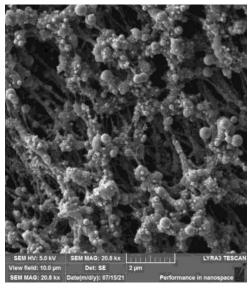
**Figure 1:** Detailed SEM image of PTFE nanotextile with sputtered Ag 300 s and subsequently treated with 150 mJ.cm<sup>-2</sup>
