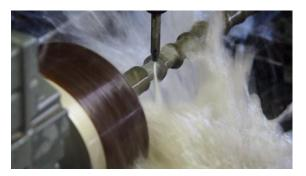
**Figure 1**: Photo of tangential abrasive waterjet turning. The deflection of the jet visible in the picture is important phenomena, which may show that the set up parameters of the machine are not able to turn material to the desired diameter. Multipass trajectory was chosen to perform the machining. Special lathe with Lenze engine was constructed and used for this purpose.
