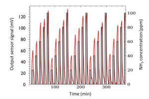
**Figure 2**: Dynamic response at room temperature of SPR sensor implementing optical grating coated by 50nm of CuPc exposed to 20, 40, 60, 80 and 100 ppm of NH<sub>3</sub>.
