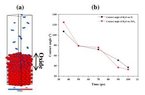
**Figure 1**: (a) Oxidation process of Ti, and (b) wettability of Ti and TiOx as a function of time.
