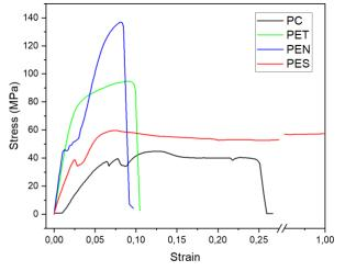
**Figure 1**: Stress – strain plot of the polymer substrates PC, PET, PEN and PES.
