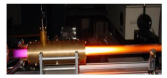
Figure 1: Nitrogen plasma afterglow
