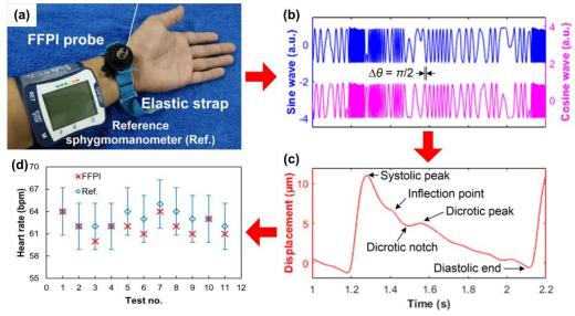
**Figure 1**: Pulse wave monitoring using a designed FFPI probe; (a) setup on a human participant, (b) interferograms from pulse monitoring, (c) demodulated pulse wave with clearly defined characteristics, (d) summarized heart rate measurement results
