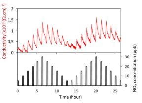
**Figure 1**: Dynamic response of phthalocyaninebased chemoresistor exposed to various concentrations of NO<sub>2</sub> in the 5-30 ppb range. Each exposure sequence consists in 15min of NO<sub>2</sub> exposure with consecutive 60min of recovery under clean air. Sensing layer thickness is 50nm, relative humidity is closed to 0.3% and the operating temperature is set to  $60^{\circ}$ C.
