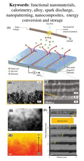
**Figure 1**: (A) Schematics of gas phase electrodeposition, (B, C) TEM/SEM micrographs, (D, E) EDX studies on a scale of 5 nm; and (F) high speed videography of selfpropagating reaction wavefront on ignition.
