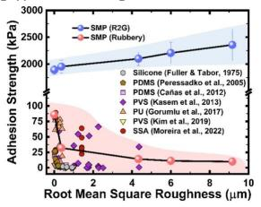
Fig. 1 Adhesion strength of SMP-based smart adhesives under R2G condition for a range of surface roughness, and comparison with other adhesive materials.
