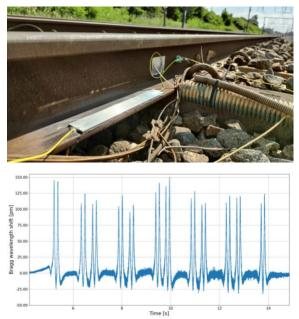
**Figure 1**: Packaged FBG strain sensors glued on the foot of the rail (top) and typical FBG response as a function of time showing the axles detection (bottom).
