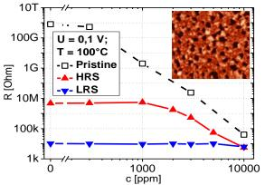
**Figure 1**: Comparison of resistances of the pristine device (dashed curve) and formed gasistor device with the memristor in the HRS (red curve) and LRS (blue curve) as a function of  $H_2$  concentration in air. The inset shows a 5×5  $\mu$ m AFM topography image of the proposed nanoporous top electrode.
