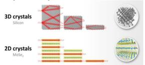
**Figure 1**: Schematic view of the heat transport mechanism in 3D materials compared to layered materials composed of 2D sheets. In the latter case, thermal conductivity is quite unsensitive to the thickness, as heat is transported within each layer.
