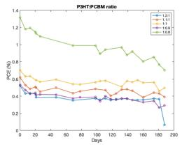
**Figure 2**: PCE decadence vs. time for different P3HT:PCBM ratios.
