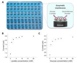
Figure 1: A) Image example of a sheet of the stretchable printed sensors and detail of the amperometry technique used to measure the concentrations of glucose and lactate. B) Amperometric lactate correlation and C) amperometric glucose correlation from 0 - 20 mM.
