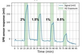
**Figure 3**: Output signal variations versus time of SPR sensor implementing 15 nm of Palladium as sensing layer coated on optical grating for various hydrogen exposure sequences in the 0,5-2% concentration range. Measurements are performed at room temperature in pure air.
