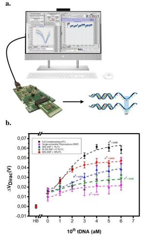
**Figure 1**: a. The microsensor is based on a graphene-FET array; b. calibration curve in phosphate buffer for mutated DNA mixed with healthy DNA (0.1:100; 1:100; 10:100).
