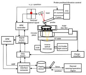
**Figure 1**: Schematic of AFM based nanorobotic system in bioorganisms measurement and manipulation.
