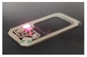
**Figure 1**: Image of the wireless-powered printed electronic circuit for the Optogenerapy implant, based on optogenetics for the treatment of Multiple Sclerosis treatment<sup>[3].</sup>
