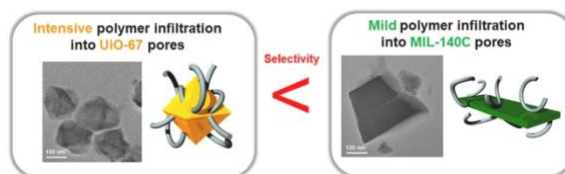
Figure 1: Figure comparing degree of polymer infiltration of UiO-67 and MIL-140C leading to different CO 2 /N 2 selectivity performance.
