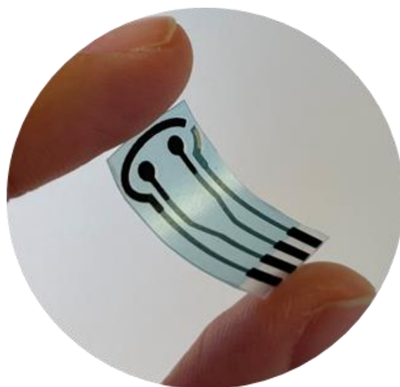
Figure 1: Printed sensor integrated on the smart patch to measure the concentrations of glucose and lactate
