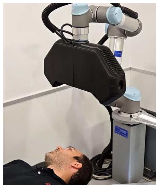
Figure 1: Figure illustrating the measurement process using the medical device developed. The head of the device integrates the luminaire, the stereoscopic sensor and the hyperspectral sensor that characterizes the area to be explored.
