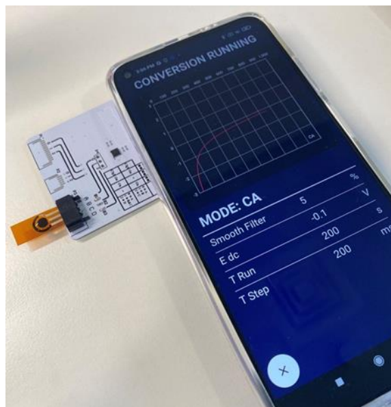
Figure 1: Digital, wireless, minimalistic, self-operated saliva glucometer developed.
