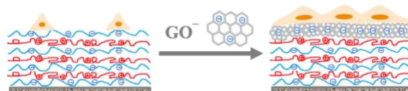
Figure 1: GO-layer promotes adhesion and proliferation of 3T3 fibroblasts and HUVEC endothelial cells on PEM-based coatings.
