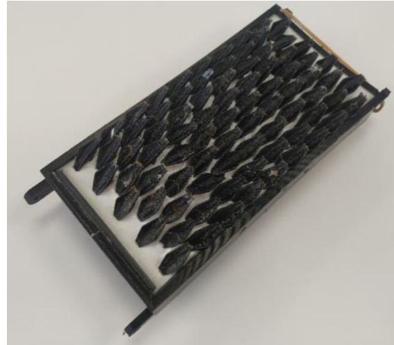
Figure 1: The figure shows one of the specimens used in the viscous drag measurement tests, where can be seen an example of a bio-inspired coating formed by multiple denticles embedded in a hydrogel substrate.
