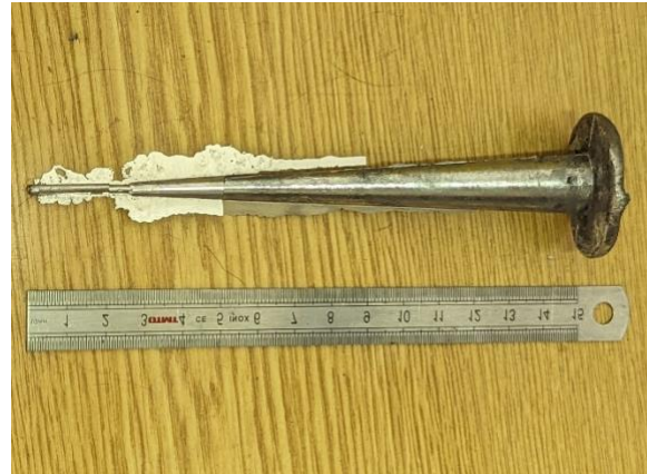
Figure 1: Image showing the Mg based bulk metallic glass produced through copper mold casting method.
