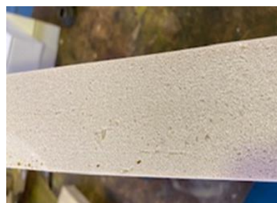
Figure 1: Cross section of hybrid epoxy/NIPU foam structural insulation panel after preparation
