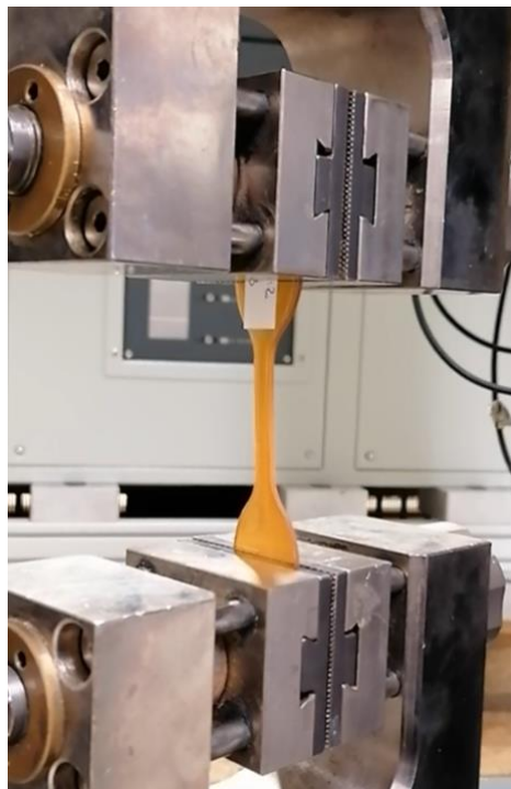
Figure 1: Tensile test of epoxidised linseed oil specimen cured with a bio-based hardener
