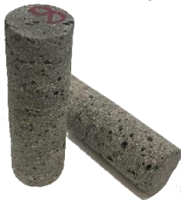
Figure 1: UHPFRC samples in shape of prisms which were subjected to dynamic testing using Split Hopkinson pressure bar.
