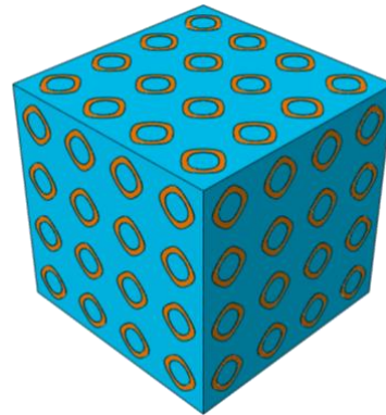
Figure 1: Figure illustrating the interpenetrating phase composites (IPCs) based on 3D printed triply periodic minimal surface structures.
