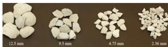
Figure 2: illustrating the shell particles of coarse aggregate sizes (12.5, 9.5, 4.75, and 2.36 mm) for use in the mixture preparation[2,3].
