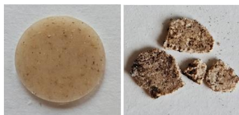
Figure 1: Figure illustrating the degradation of the PHBV composite with 2 wt.% of RS after 90 days in soil media.
