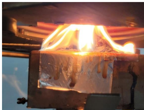
Figure 1: Fire Analysis Trial in Cone Calorimeter of Materials Resulting According to ISO5560.
