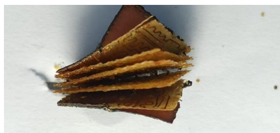
Figure 1: By dimethylsulfoxide delaminated PCB consisting of several layers of glass fabric and copper wafers bonded with epoxy resin.
