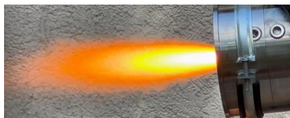
Figure 1: A schematic representation of a 100 kW steam plasma torch, showcasing the system's operation with a steam input of 10 kg/h
