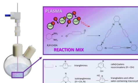
Figure 1: Graphical abstract illustrating reaction setup and the schematic representation of imine macrocycle synthesis
