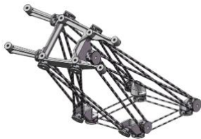
Figure 1: Figure illustrating the design of Carbon fiber / aluminium satellite Telemetry and Telecommand antenna support. This design has been manufactured with GRAM® technology and has been submitted to mechanical tests and thermos-elastic distortion tests.
