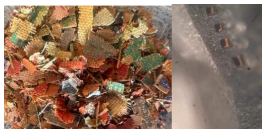
Figure 1: Figures illustrating the FR-4 residues after dissolutions of resins and hydrometalurgical extraction of metals. Gold residue is visible in the grooves of the processors plastic pieces.
