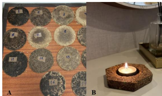
Figure 1: A – All 17 composites produced for the optimization. B - Candle holder produced by hot compression from chestnut waste with a composition of 75% chestnut, 0% glycerol at 120 °C.
