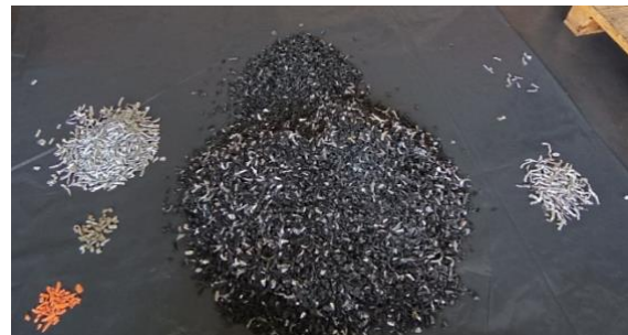
Figure 1: The image shows a shredded battery box during initial sorting to assess the components of the battery boxes and at the same time to analyze which residual materials and composites are still present after shredding the battery boxes and how they can be further processed
