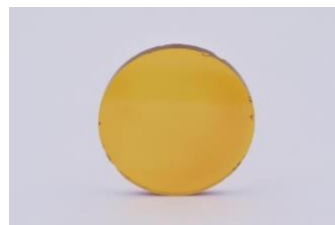
Figure 1: Optical filter of Poly(S-r-DVB) – thickness 1.6 +/- 0.02 mm
