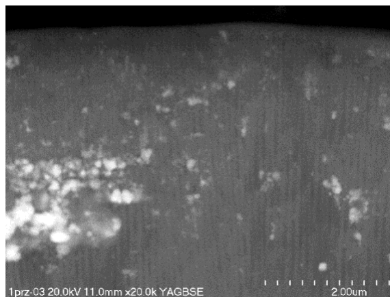
Figure 1 Fresh cross-section of the AAO coating with IF-WS 2 nanolubricant.
