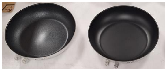
Figure 1: Two different hybrid sol-gel coating systems developed at TECNALIA and applied on Alluflon pans made with aluminium alloy AA3104.
