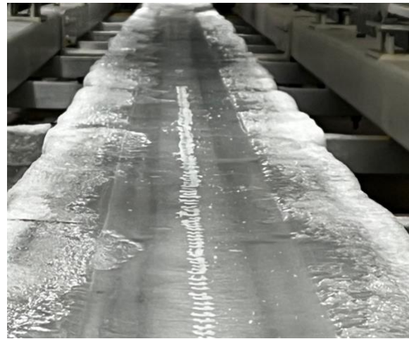
Figure 1: A machined ice track with uniformly spaced frozen water droplets offers a faster approach for testing CoF of different composition water solutions.
