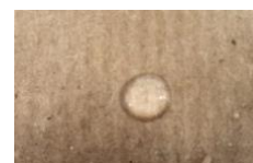
Figure 1: Water repellency on textile and packaging sector based on waterborne acrylic biobased systems.
