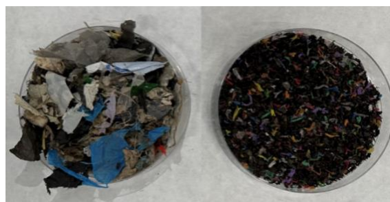
Figure 1: This image shows two samples of typical industrial plastic waste, that are used in the production of lubricating base oils. The sample on the left consists of 50% industrial plastic waste and 50% biomass, while the sample on the right is composed only with industrial plastic waste.
