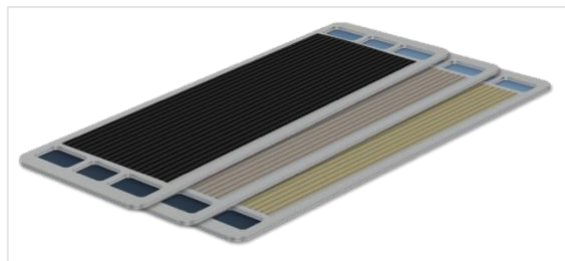
Figure 1: Figure illustrating the research topic of this study: thin-film coating development for stainless steel bipolar plates based on carbon and corrosion-resistant valve metals.
