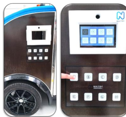
Figure 1: Autonomous electric car for last-mile delivery modified with sustainable composite car body. New flax car body part includes button panel with capacitive sensors in order to introduce the collection code.
