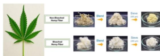
Figure 1: The physical appearances of hemp leaf and the preparation of the bleached and non-bleached hemp fiber.
