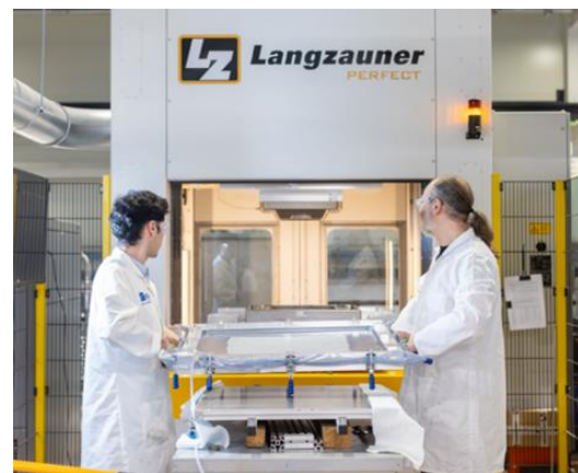
Figure 1: Manual transfer of infusion frame into press tool during in-situ polymerisation of polyamide in Double Diaphragm Forming (DDF) process.
