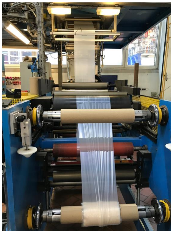
Figure 1: Film blowing process of an FDCA-based polyester blend that was developed within the Rebiolution project to demonstrate feasibility of mulch film production at an early stage.
