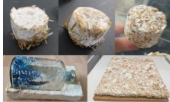
Figure 1: Figure illustrating the MBC samples prepared for mechanical and thermal testing (a)-(d); and (e) the prototype of a MBC packaging fitment for a beverage product
