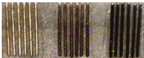
Figure 1: Textured micro-grooves on WC inserts using different laser parameters.
