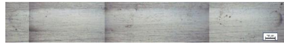
Figure 1: The friction surface of the block after the experiment with a steel ball interposed between a stainless steel pin and block (normal load: 25 N).
