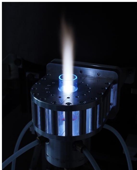
Figure 1: Microwave, atmospheric-pressure plasma torch operating with dry air used in the current work for the synthesis of NO x .
