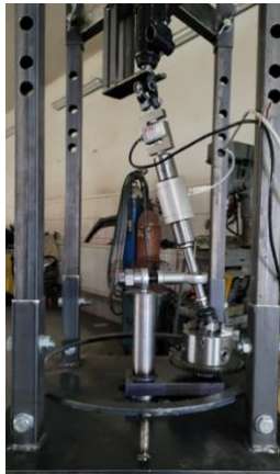
Figure 1: The tribotester equipped with a force sensor and torque meter.
