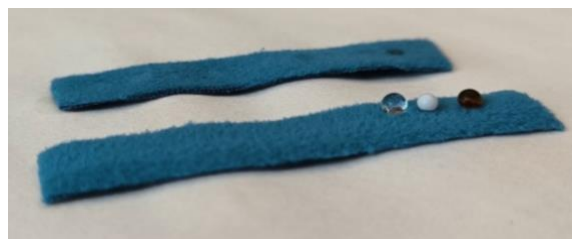
Figure 1: Water-repellent performance of plasma-coated PET textile, showing stable droplets of different liquids on the treated surface without immediate absorption.
