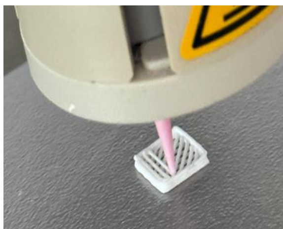
Figure 1: Additive manufacturing of baghdadite scaffolds by robocasting
