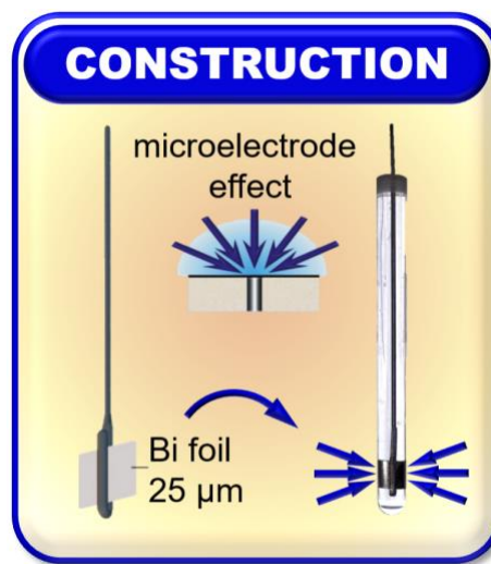
Figure 1: Schematic illustration of the bi-band microelectrode construction and operating principle. From left to right: the inner conductive core assembly showcasing the attachment of the 25 \mu\text{m} metal foil; a conceptual diagram of the microelectrode effect featuring convergent, non-planar mass transport; and a photographic view of the final assembled sensor with arrows indicating the multi-directional diffusion lines toward the symmetrically opposed microbands.
